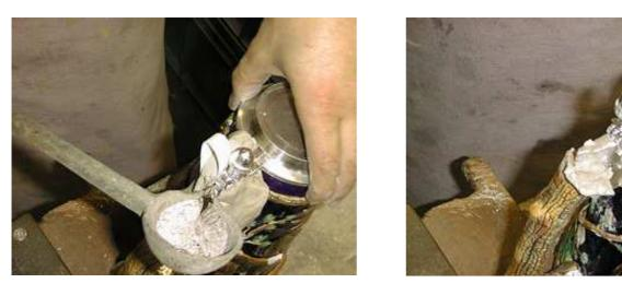
In the next step liquid pewter is poured into the artificial mold which will build a seamless connection between the lid and the handle.
