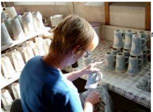
After the stein is removed from the gypsum form, craftsmen apply the base coat glaze on the stein. In nearly all instances this is a manual, very labor intensive process.
