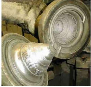
**3 Opening the mold** After the mold is cooled down, it can be opened carefully and the raw lid will be carefully removed and prepared for the next step.
