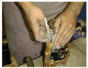
In the first two steps, a strip heat resistant material will be tied around the handle. Then everything will be covered with a heat resistant putty, which will create a mold for the lid mount.
